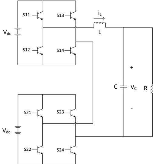
Figure 2. 5-level CHMI with LC filter
