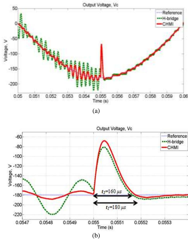
Figure 6. Comparison of output voltage waveform during no load to full load condition showing ripples and transient time,  $t_1$  and  $t_2$  (a) Ripples (b) Transient time
