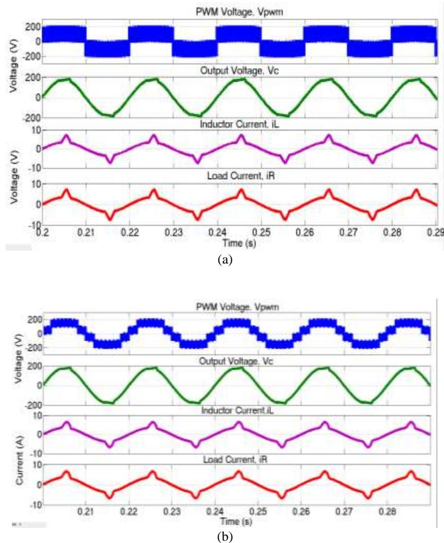
Figure 9. System response structural uncertainty, top to bottom, PWM voltage  $V_{PWM}$ , output capacitor voltage  $v_C$ , inductor current  $i_L$ , and load current  $i_R$  (a) H-bridge Inverter and (b) 5-level CHMI
