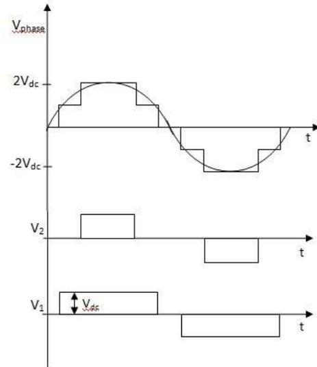
Figure 3. 5-level CHMI output voltage waveform
